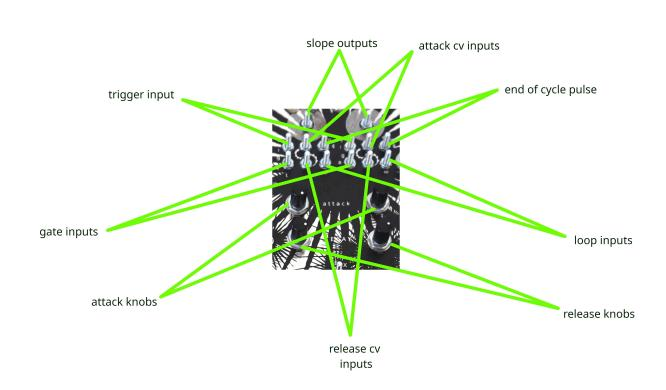
THE TWO SLOPES HAVE 2 KNOBS EACH. THE UPPER ROW OF KNOBS CONTROLS ATTACK TIME OF EACH RESPECTIVE SLOPE. THE BOTTOM ROW OF KNOBS CONTROL DECAY TIME FOR EACH SLOPE.
