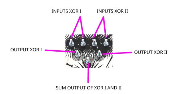
TECHNICALLY SPEAKING, AN XOR GATE OUTPUTS THE DIFFERENCE OF 2 LOGIC SIGNALS. MEANING THAT IT OUTPUTS A LOGIC 1 ONLY WHEN 1 INPUT IS AT LOGIC 0 AND 1 INPUT IS AT LOGIC 1
