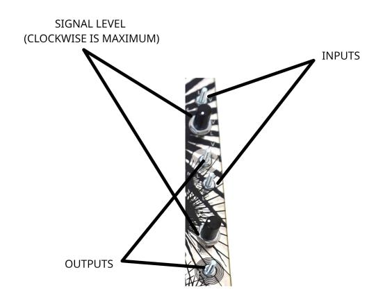
THE TWO ATTENUATORS OR LEVEL SHIFTERS ARE LOCATED AT THE FAR RIGHT OF THE PANEL IN A VERTICAL COLUMN AND ARE REPRESENTED BY 1 KNOB AND 2 PATCHPOINTS EACH. THESE ARE SIMPLE UTILITY MODULES THAT GREATLY EXPAND ON THE POSSIBILITIES OF THE EACH OF THE OTHER MODULES.
