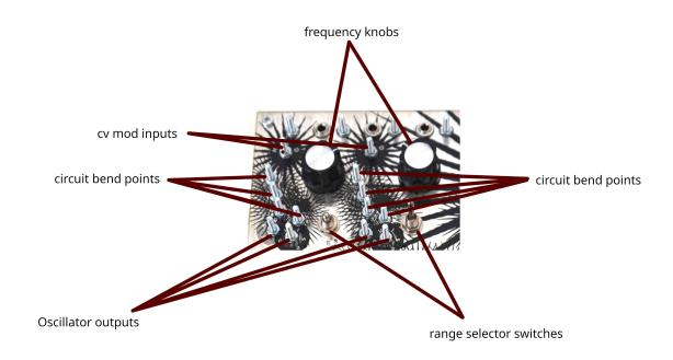
THE 2 VCO OSCILLATORS HAVE 1 SWITCH EACH THAT SELECTS THE COARSE OSCILLATION RANGE. MIDDLE POSITION OFFERS FULL AUDIO RANGE, UPWARD POSITION PRESENTS BASS AUDIO RANGE, AND DOWNWARD POSITION IS SUB AUDIO LFO RANGE.
