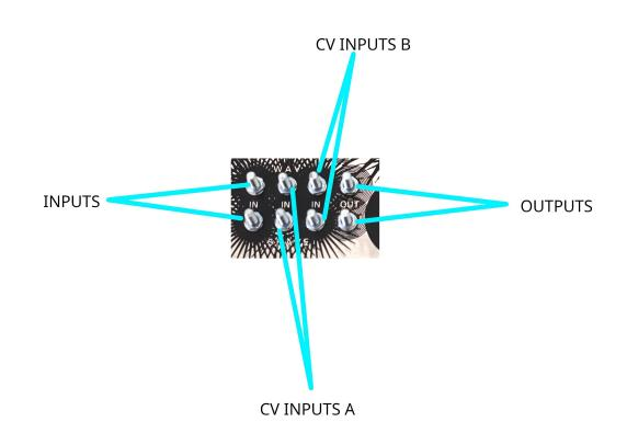
UNDERNEATH THE NOISE SECTION, AND JUST TO THE RIGHT OF THE LOW PASS GATE, IN THE BOTTOM LEFT OF THE PANEL OCCUPYING 2 HORIZONTAL ROWS THERE ARE THE 2 WAVESHAPERS.
