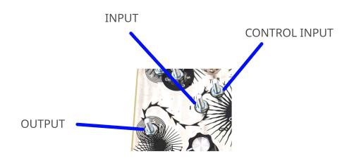
THE HIGH PASS GATE CAN BE USED TO GATE SIGNALS- GOOD FOR CREATING PERCUSSIONS IN THE UPPER FREQUENCY RANGES.
