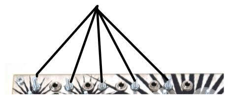
THE 5 ASSIGNABLE INPUTS / OUTPUTS AT THE TOP OF THE PANEL ARE THE HEART OF INTERFACING ANTIRAVE WITH OTHER EQUIPMENT. THIS MIGHT BE TO SEND OR RECEIVE VOLTAGES, GATES, OR AUDIO.
