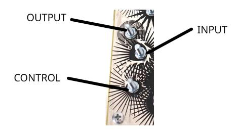
THE LOW PASS GATE CAN BE USED FOR GATING SIGNALS AND CREATES A SUBTLE LOW PASS FILTER WHICH BECOMES LOWER IN FREQUENCY AS THE GATE CLOSES.
