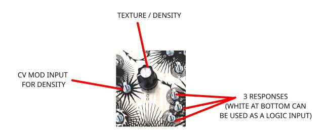
THE NOISE SECTION FEATURES 3 DIFFERENT NOISE RESPONSES WITH VARYING INTENSITIES AND FREQUENCIES. THE UPPER TWO PATCHPOINTS - VIOLET AND BLUE - ARE FILTERED AND QUIETER, SUITABLE FOR PASSIVE MIXING WITH OTHER SOUND SOURCES. WHITE IS FULL SPECTRUM AND INTENSITY AND CAN ALSO BE USED AS A CONTROL VOLTAGE OR A LOGIC INPUT.
